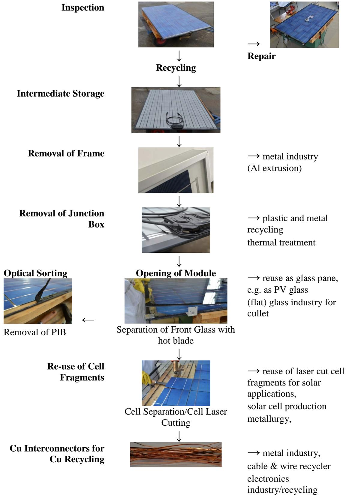
**Figure 2.1:** NICE Module Recycling
