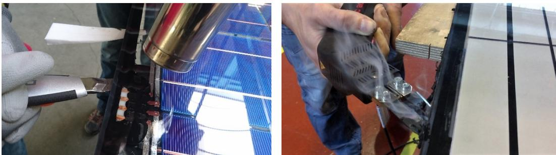
Figure 1: Opening of NICE module by hot air gun + cutter (left) or thermocutter (right)
