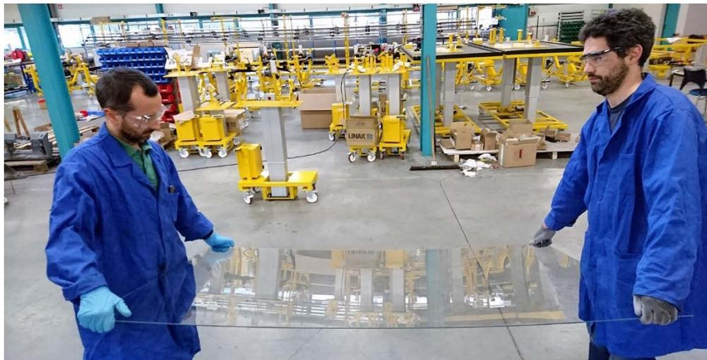
*Figure 3: Recovered glass from an old 60 cells NICE module for reuse.*
