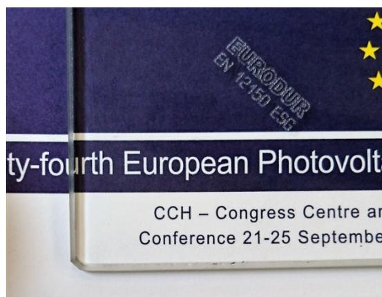
*Figure 4: Detailed view on an edge of one of the recovered glasses from old NICE modules for reuse.*
