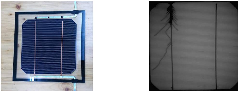
*Figure 10: One-cell NICE mini module with integrated recovered Cu-connectors from old NICE modules. Visual image on the left and EL Image on the right.*
