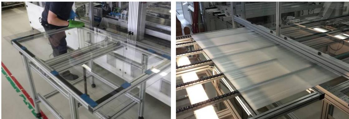
*Figure 6: Manufacturing of Glass/Backsheet modules using recovered front glass from old Apollon Solar NICE modules: Step 1 - manual glass cleaning (left) and Step 2 – laying of the front EVA sheet (right).*
