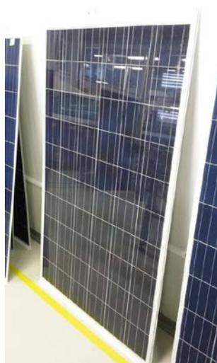
*Figure 9: Finalised glass/backsheet modules with reused front glass sheets from old NICE modules.*
