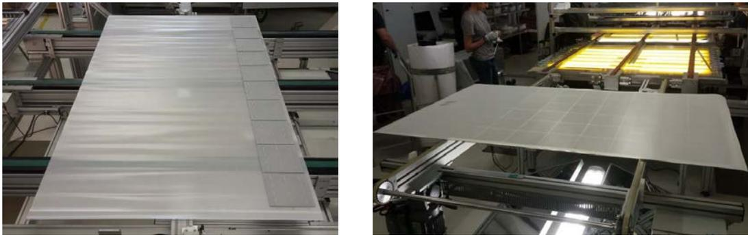
*Figure 7: Manufacturing of Glass/Backsheet modules using recovered front glass from old Apollon Solar NICE modules: Step 3 – Solar cell stringing and placing on front EVA/Glass (left) and Step 4 – interconnection and laying of 2nd EVA layer and backsheet (right).*
