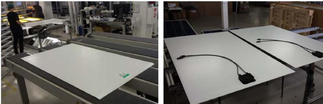
*Figure 8: Manufacturing of Glass/Backsheet modules using recovered front glass from old Apollon Solar NICE modules: Step 5 – Entering the laminator (left) and Step 6 – J-Box assembly + IV Testing (right).*
