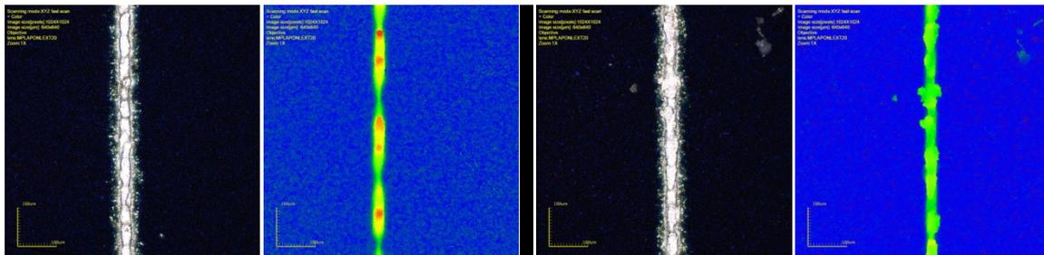
Figure 7: Color microscopy and laser scanning profile image of mc-reference (left) and of the fineline print-on-print (right).
