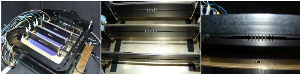
Figure 4: Left measurement setup top view with cell. Middle measurement setup without cell. Brass base chuck has insulated voltage extraction. Right side view on the top measuring bar featuring springs to ensure a defined pressure on front side metallization.
