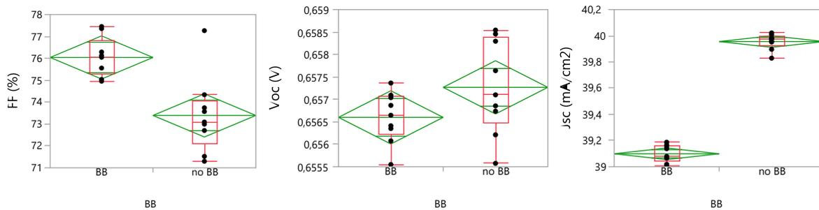
Figure 6: Measurement of BiSoN cells without BB using the no BB measuring chuck.
