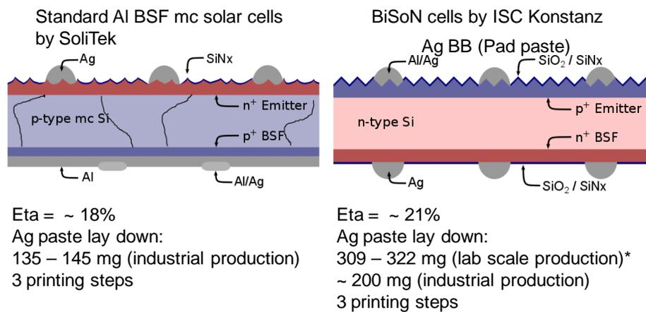
Figure 3: mc solar cell and BiSoN scheme and metallization overview. Note: Ag/Al paste means that a small fraction of Al is added to the silver paste for improve contacting for  $p^+$  structure
