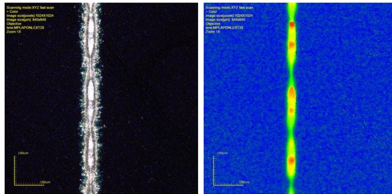
Figure 2: Optical and laser scanning microscope image of a fineline printed finger (single print).
