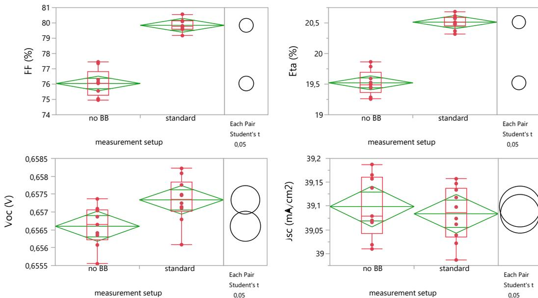
Figure 5: Measurement of BiSoN cells with additional BB using the two possible measurement setups.
