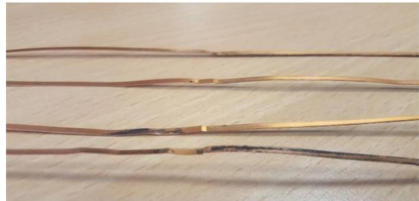
Fig. 3. Recovered copper tabs from discarded NICE modules.
