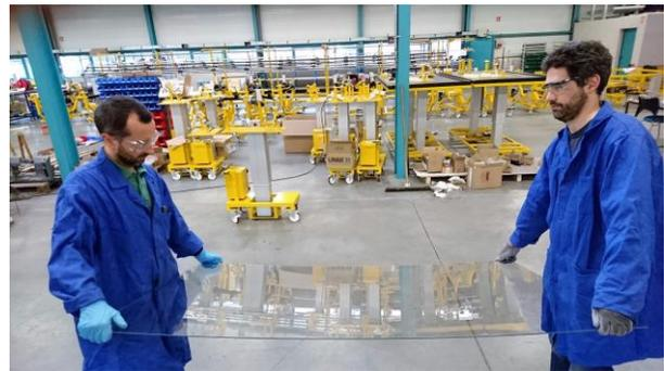
Fig. 2. Recovered front glass from a disassembled NICE module
