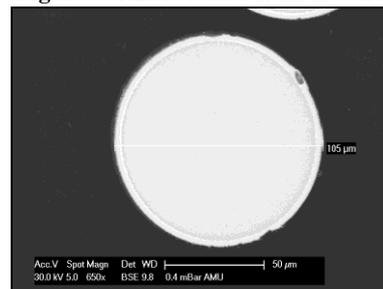
**Figure 4:** REM cross section of used diamond wire
