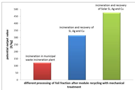
**Figure 5:** Potential material values after different recycling processes of PV modules
