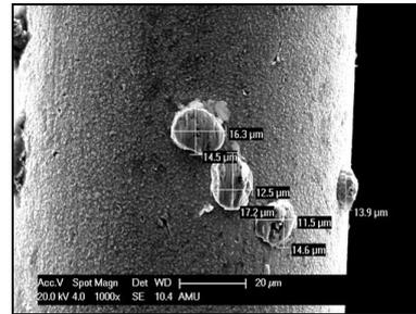
**Figure 1:** REM of new diamond wire
