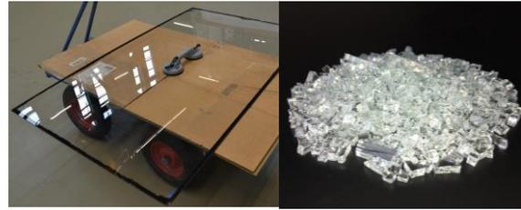
**Picture 9 and 10: Glass sheet (left)/cullet (right) glass recycling, building industry**
