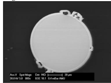
**Figure 2:** REM cross section of new diamond wire
