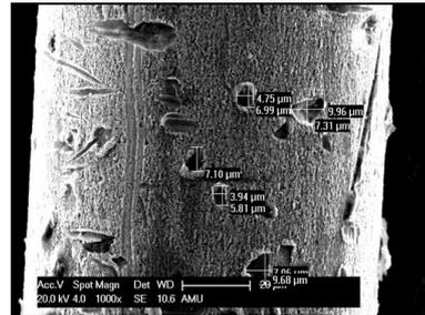
**Figure 3:** REM of used diamond wire
