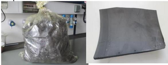
**Picture 7: Wafer sawing slurry possibly containing diamonds** metallurgy, metal recycling, organic chemistry (additives), production of abrasives, sawing wire industry, tool industry
