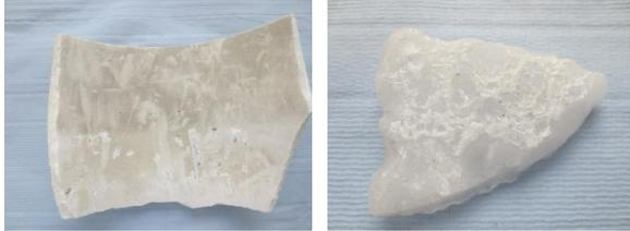
**Picture 1 and 2: Silica (left)/quartz (right) crucibles** ceramic/glass industry, horticulture, building industry, production of abrasives, ferrosilicon production, additives for dispersions/polymers
